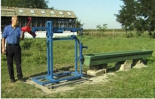
Figure 3. A hand water pump with a pendulum in a field (vicinity of Novi Sad, August 2004) http://youtu.be/hNpql7o_1QI
