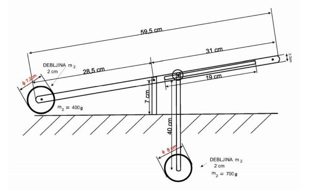
VEMIRC Pendulum Lab © 2012 Veljko Milkovic Research & Development Center www.pendulum-lever.com | www.veljkomilkovic.com Dimensions and Weights of Veljko Milkovic's Two-Stage Oscillator Table Models
